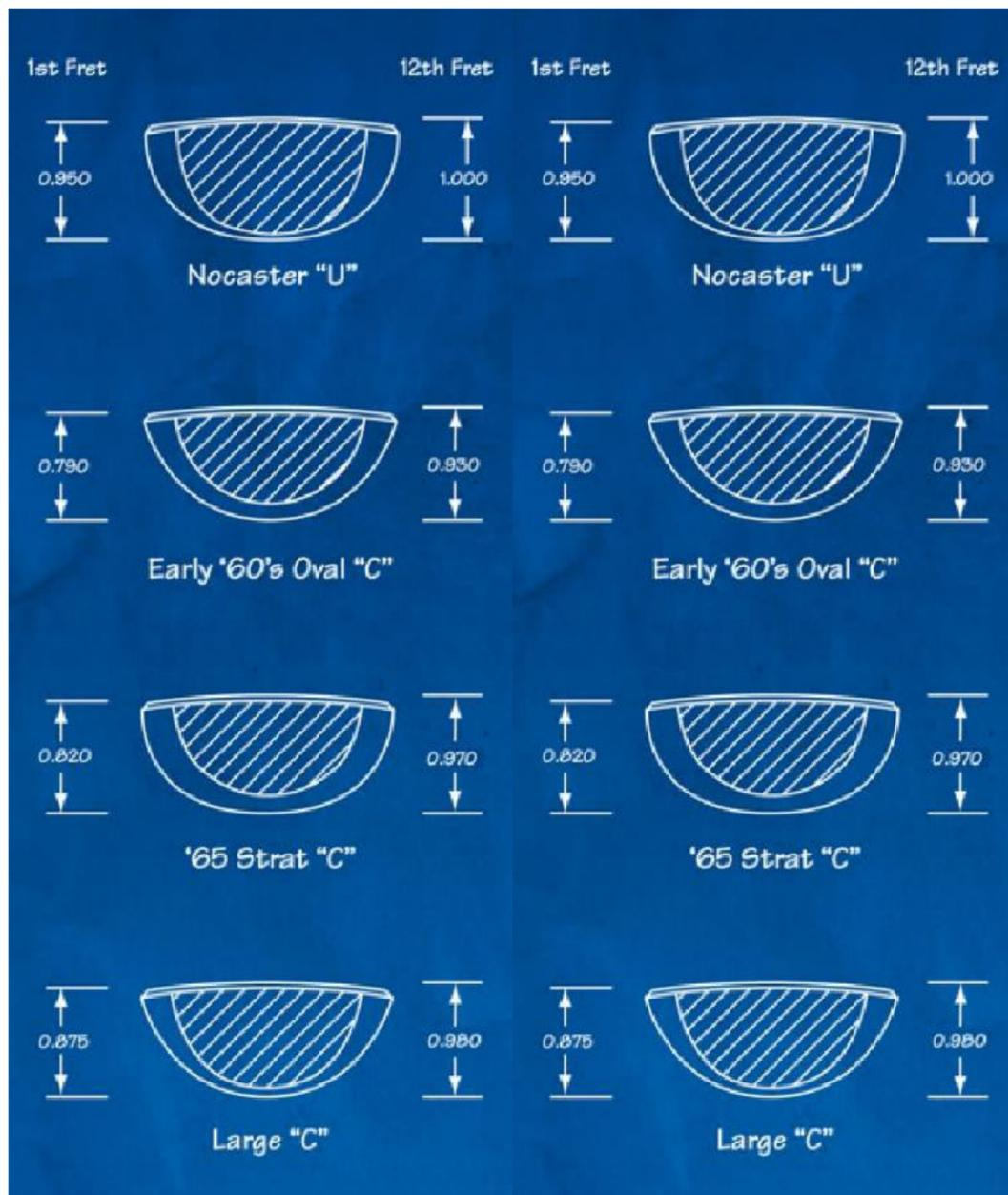
GUITAR AND BASS NECK PROFILES FOR MAKING TEMPLATES. PRINT THEN GLUE TO 1/4" MDF. USE ONE SIDE TO CUT THE 1ST FRET PROFILE AND THE OTHER SIDE TO CUT THE 12TH FRET PROFILE. FILE AND SAND TO DESIRED FINAL SHAPE.
